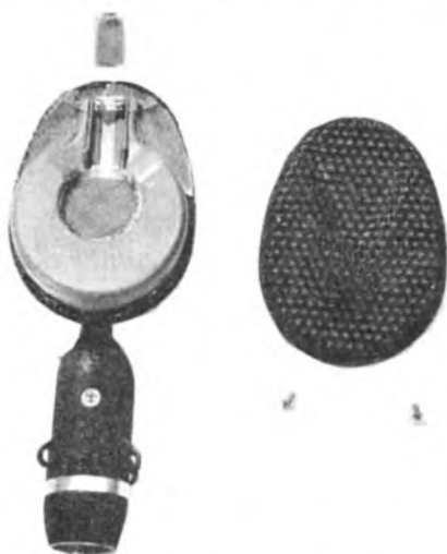
Fig. 1. The STC4038 ribbon microphone which has a "figure-of-eight" polar diagram.
